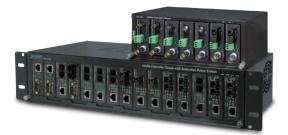
Offering more capacity to the converters in one chassis, PLANET MC-700/MC-1500 provides 7/15 slots in the 10"-19" rack saving more spaces for fiber-optic wiring yet simplifying the maintenance of media conversion. It allows the connectivity of up to 7-/15-slot PLANET Fast Ethernet, Gigabit Ethernet or VDSL2 Converters in one chassis. One fan with LED indicators for the system cooling is also available.
