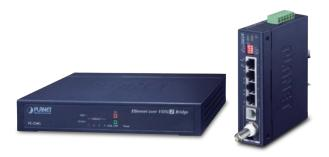
PLANET VC series is Ethernet-over-VDSL2 Media Converter with high performance. It is based on two core networking technologies, Ethernet and VDSL2 (Very-high datarate Digital Subscriber Line 2). The VDSL2 technology offers the absolutely fastest data transmission speeds over the existing copper telephone lines without the need of rewiring.
